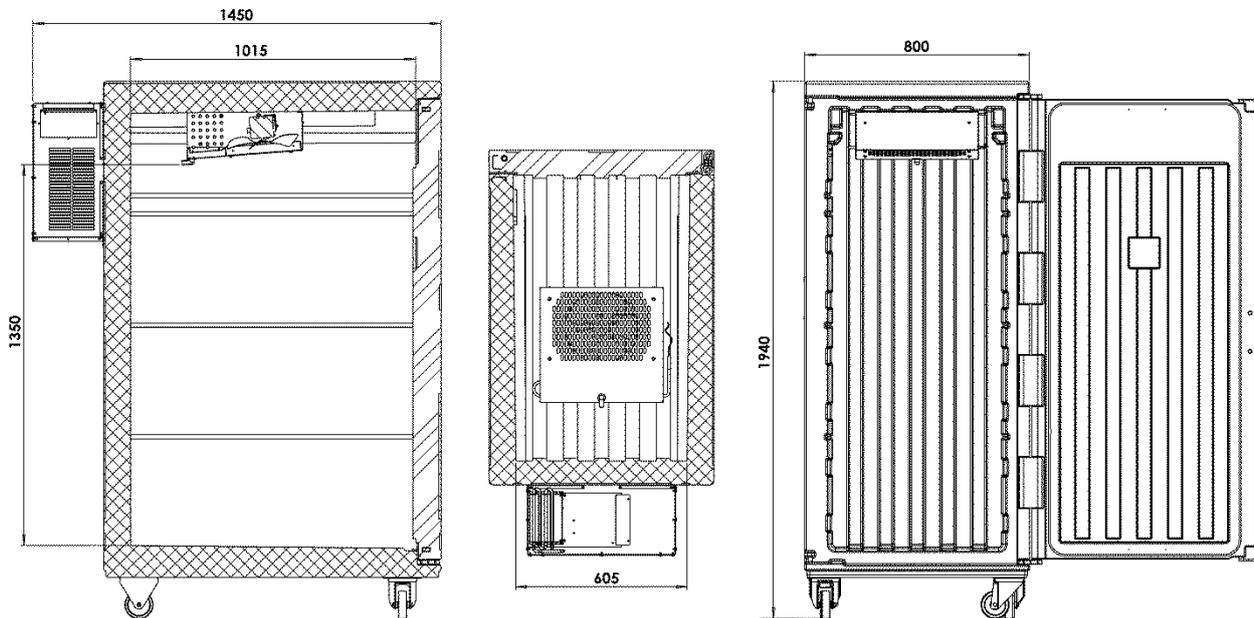
**Model with cooling unit on back ventilated**
