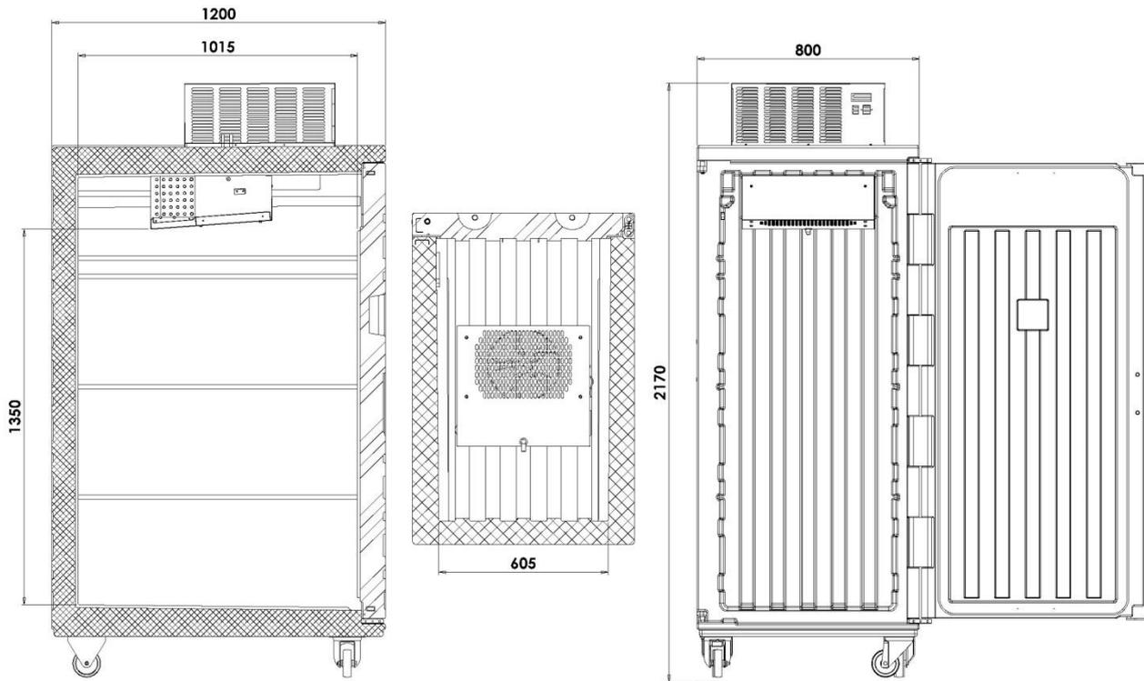
**Model with cooling unit on top ventilated**
