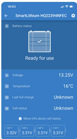
The screen will then connect to the device (in this case, the battery) and display all the essential data.
