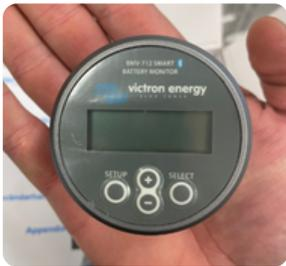
The BMV (Battery Monitor) is typically mounted on the bulkhead behind the driver. However, it is also accessible through the app.
